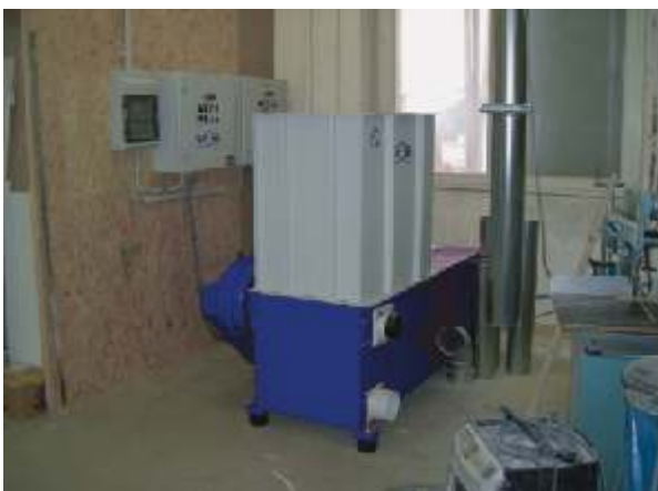
GAZ 62 shredder connected to an air suction system
